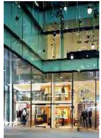
One hour fire rated, butt glazed wall system by Vetrotech Saint-Gobain. Includes entry door option.
